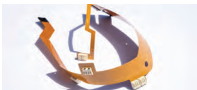
Single Sided FLEX PCB copper accessible for both side, soldered with special connectors flex to wire for battery pack interconnection
