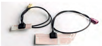
Antennas AM-FM-DAB-Wifi-Thelephony, produced in PI-Pen, soldered with components and coaxial cable, protected in accordance to IP65 by molding with hot melt or UV resin
