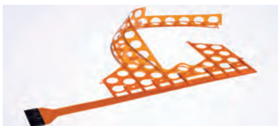
FLEX PCB n°1 layer: accessible on both side Bus bar connections
