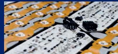
ALU FLEX PCB with SMD components for Rear Lamp
