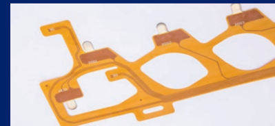
FLEX PCB single layer, length 1100 mm. soldered with NTC and Nickel Tabs
