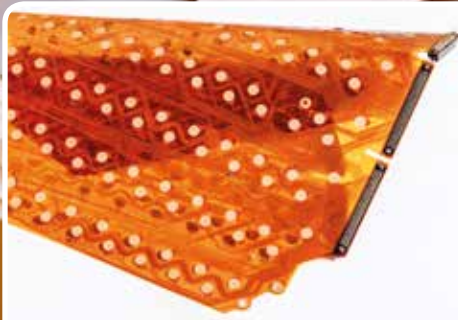
FLEX PCB Double Side copper, with soldered NTC, tabs obtained by copper open top and bottom side, THT connectors
